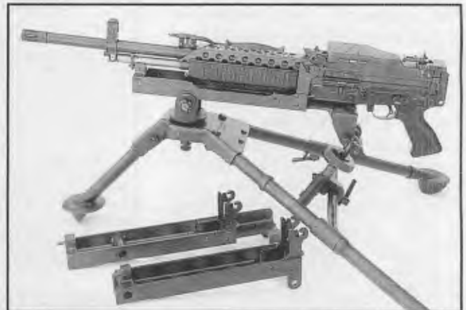
When fired off the tripod the Stoner 63A machine gun exhibits exceptional accuracy potential with a very small group dispersion. This Stoner 63A with right-hand feed and bottom cocking has been mounted on a M2/M122 BMG tripod with one of three different cradle adapters made for this purpose. Photo: Peter G. Kokalis
